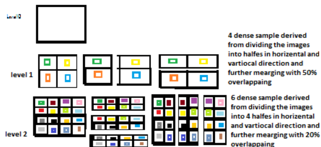
Figure 6: Example of the spatial plane division of the image into dense sampling.
